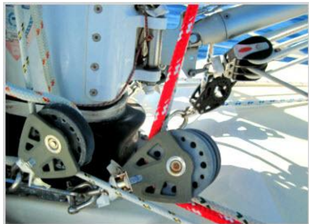
Inspect exit blocks near the base of a mast for chafe near the block where the line leads aft to the cockpit.
